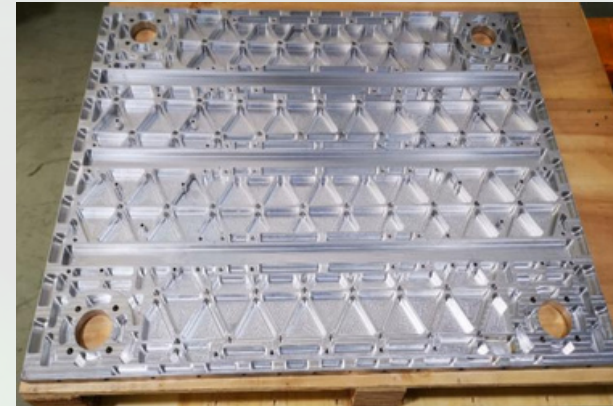
Machined Plate for Satellite telecom High tolerances Size: 1016*750*18mm Material:AL7075
