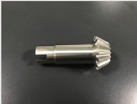
Complicated Gear with 0.005mm tolerance
